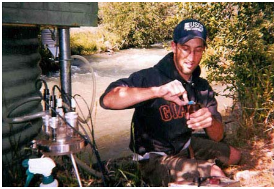
Adam Weinberg '04 acidifying a Red River water sample in Red River, New Mexico
